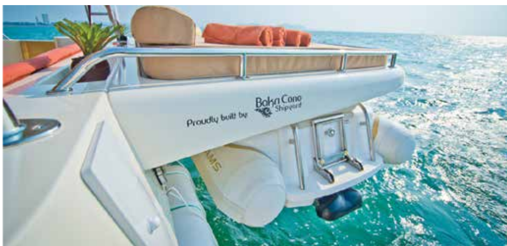
Stern platform with tender protected from weathering
